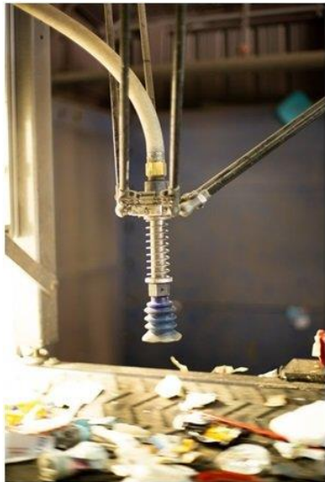
AMP Cortex™ - A robotics system that performs tasks of sorting, picking and placing material
