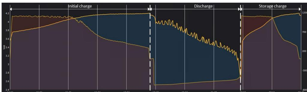
**Figure 4.** Voltage [blue] - Current [red] plot during a capacity-test. The cell-under-test is a LG MH1 of 3.200 mAh, tested by a MegaCellCharger charger.
