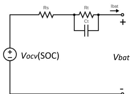
**Figure 3.** Thevenin-Based electrical model for a Li-Ion cell, with a series resistor  $R_s$ , an RC network ( $R_t$ ,  $C_t$ ) to describe basic charge transfer phenomenon, and an open circuit voltage dependent on the SOC  $V_{ocv}$  [9].
