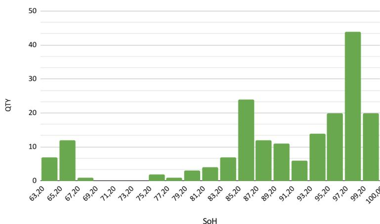
**Figure 5.** SoH of the tested cells taken from different e-bike batteries.
